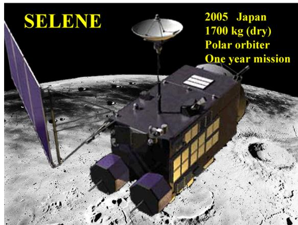
Fig. 1. SELENE (SELenological and ENgineering Explorer) Configuration. The SELENE will be launched in 2005 by H-IIA rocket of NASDA. It is a 2-ton-class explorer. It will investigate the Moon by 15 mission instruments.
