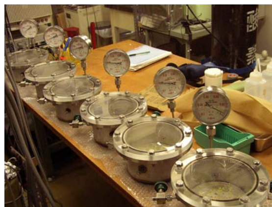
Figure 1. Picture of the experiment equipment. The cultivation vessel made of stainless with pressure gage and window for observation.
